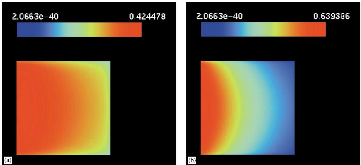
Fig. 9. (a) and (b) show the mean, angle-averaged intensity for the pure scattering problems where  $\varepsilon = 0.3$  and  $\sigma = 5$  and 25, respectively.  $96 \times 96$  mesh points along with the  $S_6$  LSH ordinate set were used.
