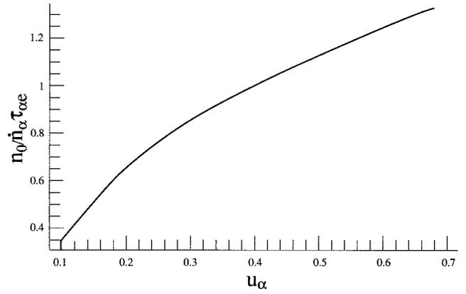
FIG. 15. Normalized density of thermonuclear  $\alpha$  particles in a plasma with  $1 \leq T \leq 50$  keV with an initial creation speed  $v_{\alpha} = 1.3 \times 10^9$  cm/s.
