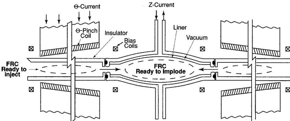
FIG. 2. Field reversed configuration (FRC) plasma in implosion geometry [R. E. Siemon, I. R. Lindemuth, and K. F. Schoenberg, Ref. 1, p. H 1].
