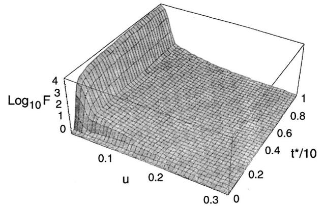
FIG. 12. Temporal evolution of the  $\alpha$  distribution ( $E_\alpha=3.5$  MeV), plasma temperature  $T=5$  keV  $\Rightarrow u_\alpha=0.308$ .
