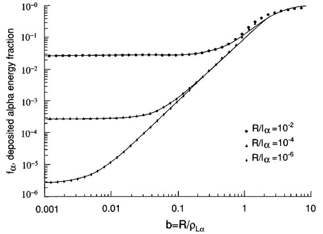
FIG. 3. The energy fraction  $f_\alpha$ , which the 3.5 MeV alpha particles deposit in a uniform magnetized DT cylinder, as calculated by performing numerical integration in Eq. (7) (dots, triangles, and diamonds). Approximate formula (12) is plotted with the solid curves. The three curves display the dependence of  $f_\alpha$  on the dimensionless parameter  $c$  for three different values of  $\bar{R}$  [see Eq. (2)].
