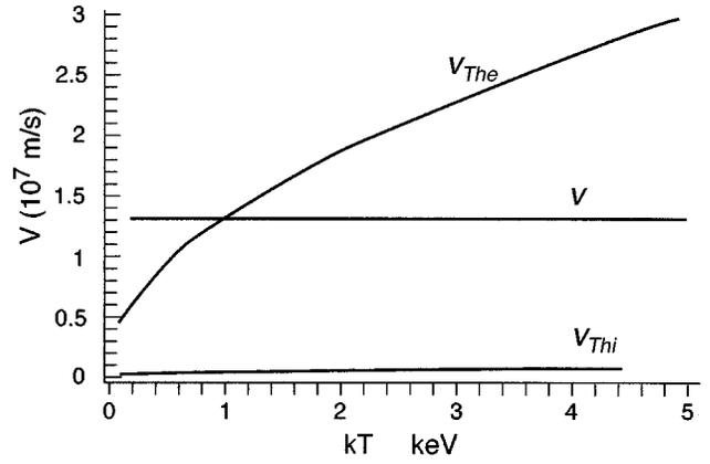
FIG. 5. Mean initial  $\alpha$ -particle velocity  $v$  contrasted to  $v_{The}$  and  $v_{Thi}$  in terms of  $T = T_e = T_i$ .
