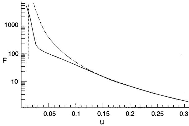
FIG. 11. Full equilibrium distribution (78) (continuous line) for thermonuclear  $\alpha$  particles and its approximation (82) (dotted line)  $T=5$  keV,  $u_\alpha=0.308$ .
