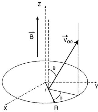
FIG. 1. The coordinate system used in Sec. II for calculating the alpha energy deposition fraction  $f_\alpha$ .
